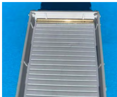
Inside of wagon showing the length of bullhead rail across the end, covering the strapping.
