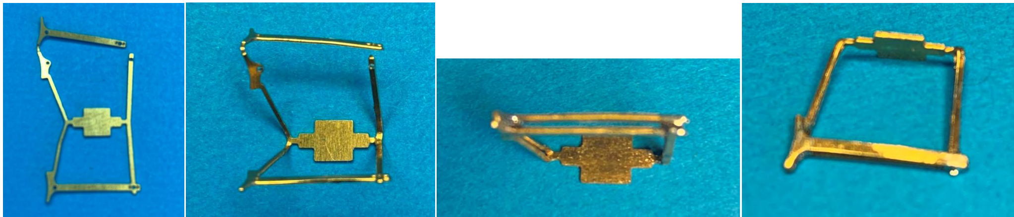
Stages of folding and assembling the brake shoes
